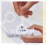
After the specified reaction time of at most one minute has expired, the color of the reaction zone is compared with the color scale printed on the tube label and the corresponding concentration is read off.
