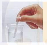
The reaction zones are wetted with the solution to be tested simply by dipping them briefly into the liquid sample. Any excess liquid is then shaken off or removed by drawing the test strip across the edge of the vessel.
