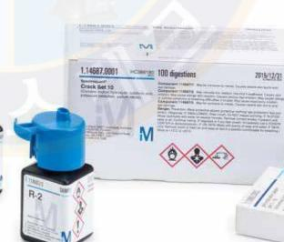
When the objective is to determine the total content of certain parameters, the Crack Sets contain all the necessary reagents.
